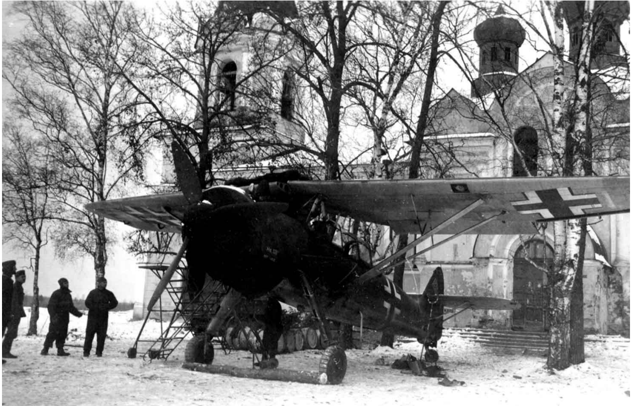
Luftwaffe groundcrew prepare to move a two-seater Henschel Hs 126 reconnaissance aircraft to safety. Just over 600 of these aircraft were built but they were progressively replaced from 1942 by the twin-engine Focke-Wulf Fw 189.
