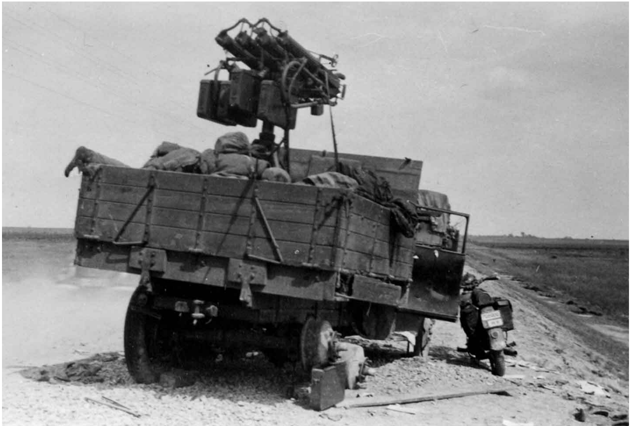
A Soviet truck mounting heavy machine guns used in an anti-aircraft role.
