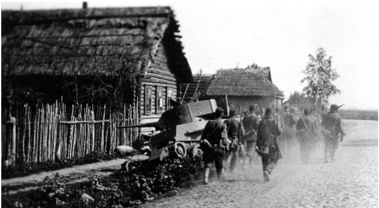
German troops file past an abandoned B-5 fast tank. This design went into production in Kharkov in the mid-1930s. It was followed by the improved BT-7, identifiable by its conical (rather than cylindrical) turret. Both were superseded by the T-34.
