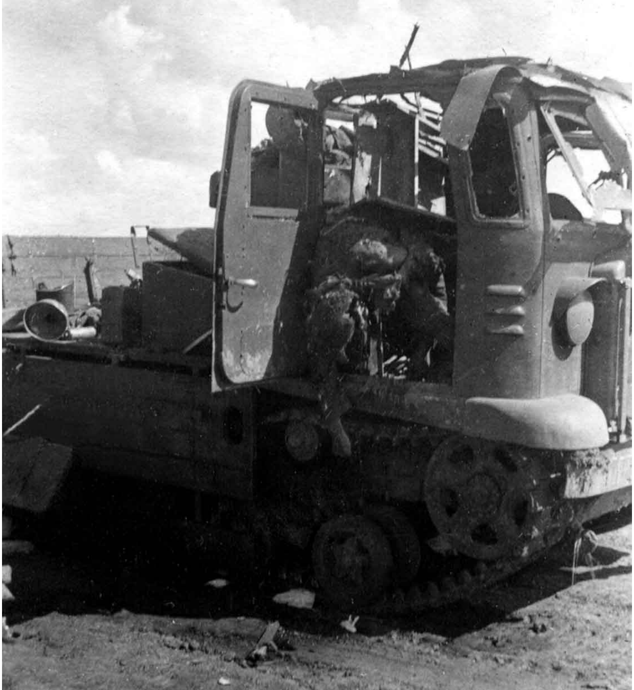
The remains of a Soviet STZ-5-2TB tracked prime mover used to tow artillery. The Germans employed captured examples as the Artillerie Schlepper CT3-601(r).
